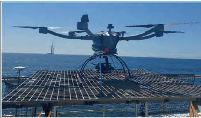
Figure 9.10. RAVEN UAV developed for ATLANTIS (developed by INESC TEC).
