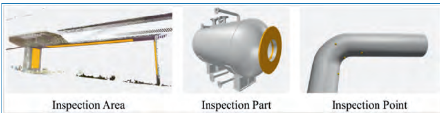
Figure 6.8. Examples of different inspection locations on the IVP: pillars and deck of a viaduct, depicted as bounding boxes on the asset surface (left); the nozzle of a pressure vessel, highlighted in orange (center); specific points of a pipe, depicted as small spheres (right).
