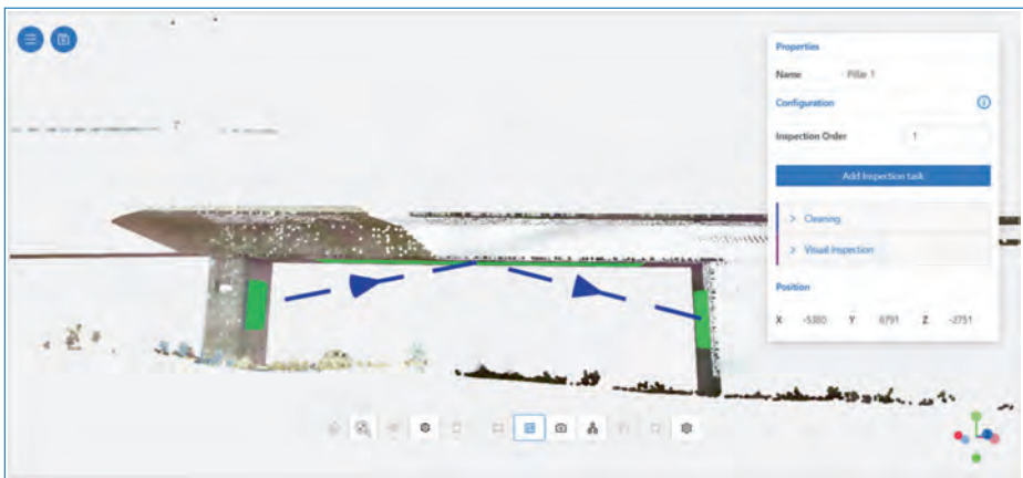
Figure 6.10. Example of the inspection tasks 3D editor. Inspection locations allow task additions with few simple clicks, turning them green once tasks are assigned. The blue arrows indicate the robot inspection-sequence: starting with the left pillar, moving to the deck, and concluding with the right pillar.
