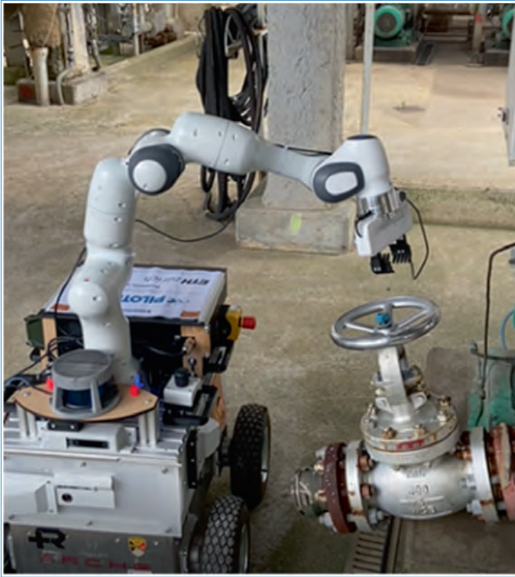
Figure 7.2. Image of the UGV equipped with a manipulator. The inspection plan provides the location of the asset in the pre-built map, then the UGV localizes within the same and navigates towards the asset's location and proceeds with the manipulation.
