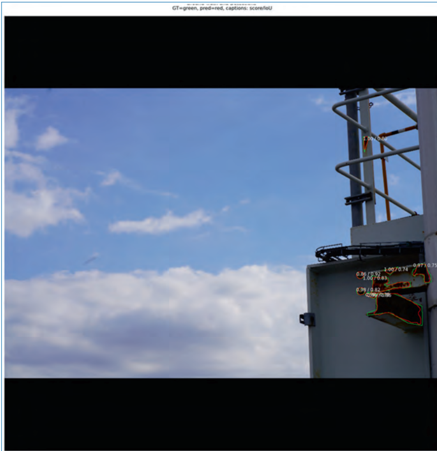
Figure 3.15. Sample image predictions on the test set using MaskRCNN. Green is the ground truth annotation, red is the prediction. Next to each annotation there is the confidence/IoU.
