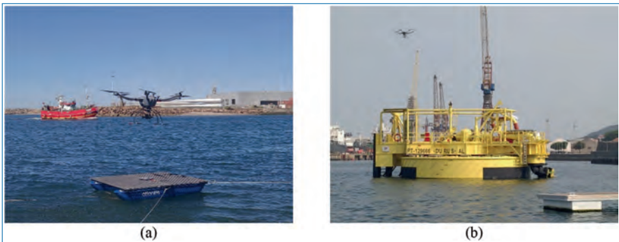
Figure 9.13. RAVEN UAV landing autonomously on the NEST landing platform (a) and on the DURIUS (b).
