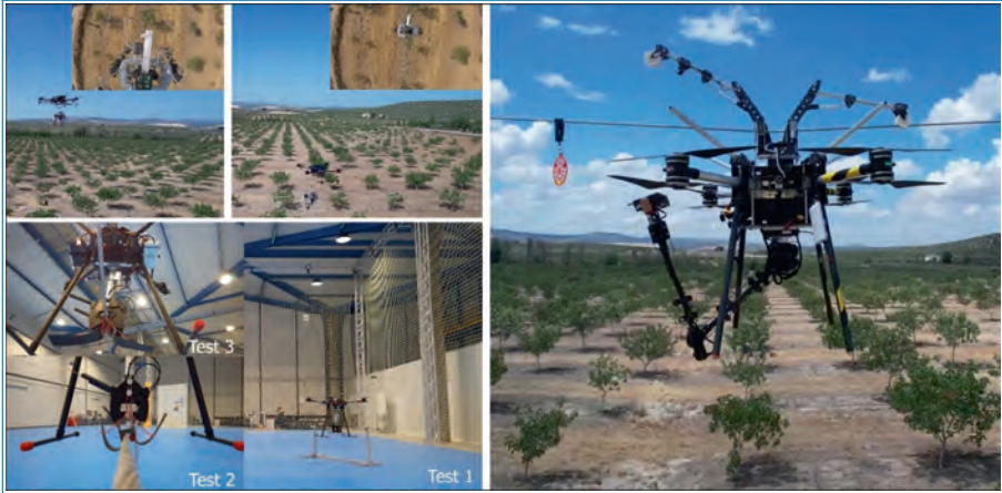
Figure 8.3. Linear Actuator Platform (LAP, up-left), Dual Arm Platform with Cart (DAP-C, down-left), and Main Local Manipulation Platform (MLMP, right) developed as part of the AERIAL-CORE project.
