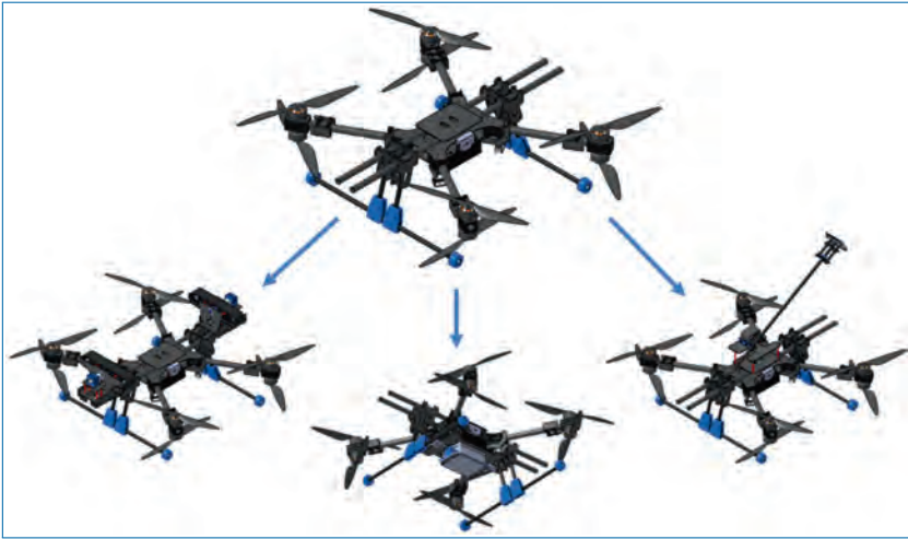
Figure 5.7. VIAD-DRONE modular concept.
