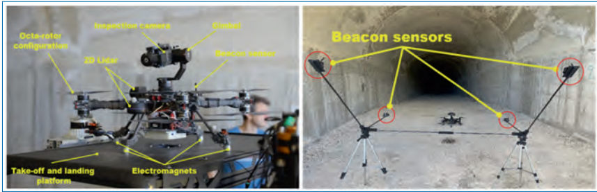
Figure 5.14. TTDRONE hardware setup used (left) and the 3D printed structure built (right) for the Scenario 1 experiments.
