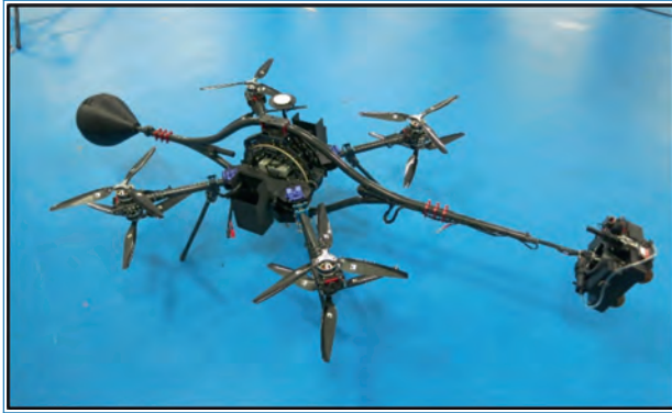
Figure 5.1. AeroX version 3 aerial robot.
