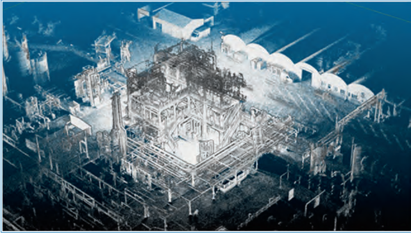
Figure 7.1. Image of a pre-built map for missions in a refinery environment, recorded using a single Ouster OS1-64 LiDAR sensor and its integrated IMU.
