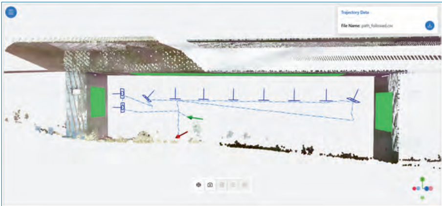
Figure 6.12. Drone trajectory overlaid on a digital twin of a viaduct, depicting the exact flight path the drone undertook during the inspection.
