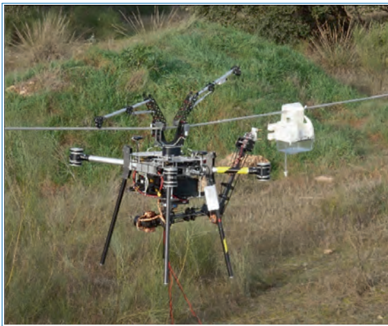
Figure 8.6. MLMP using the robotic arm to charge its batteries from a drone charging station on a controlled environment.
