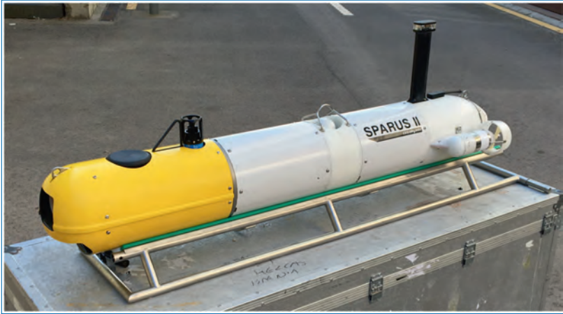
Figure 9.18. The designed docking payload integrated in the Sparus II platform (developed by UdG and IQUA Robotics).
