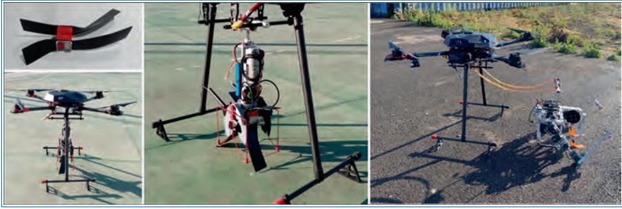
Figure 8.5. Linear Actuator Platform (left and middle) used for the installation of clip-type bird flight diverters (up-left), and Dual Arm Platform with Cart (right) for its deployment on the power line and installation of customized clip-type bird diverters.
