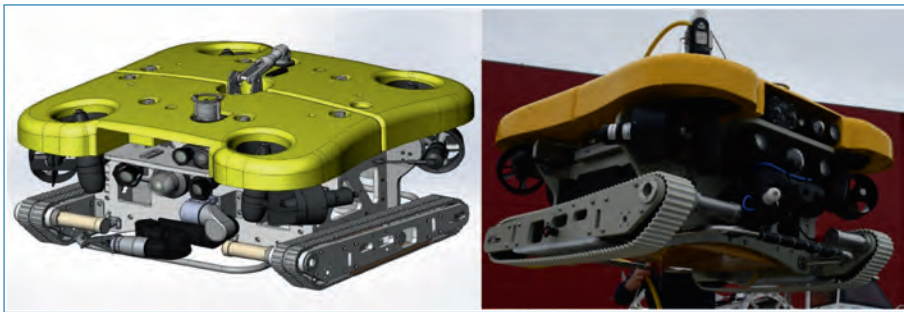
Figure 9.24. Design of the Roving Bat (left) and final system deployed (right) (developed by Exail).
