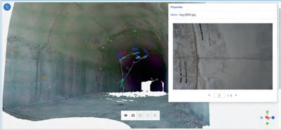
Figure 6.13. 3D visualization of inspection images. Blue markers with arrows indicate the specific asset regions represented by each image, while the violet highlight identifies the image currently displayed in the “Properties” card.
