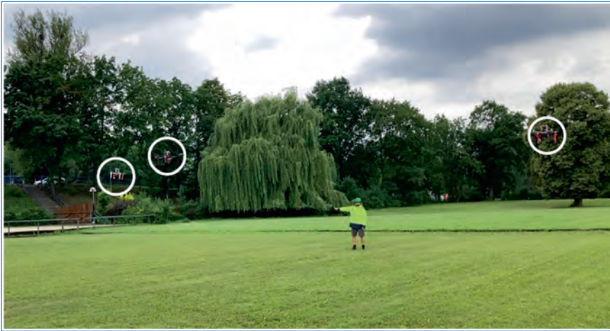
Figure 8.12. Real demonstration of team of three Safety-ACWs controlled by gestures of the human worker.
