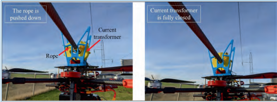
Figure 8.8. An optimized grasping system with only one current transformer [27].
