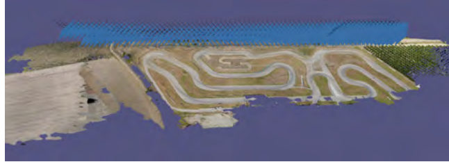
Fig. 3. Digital model generation process, the blue rectangles represent each acquired image
