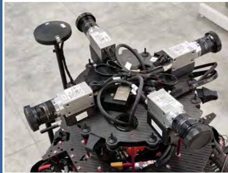
Fig. 5. Detail of the detection and avoidance system cameras
