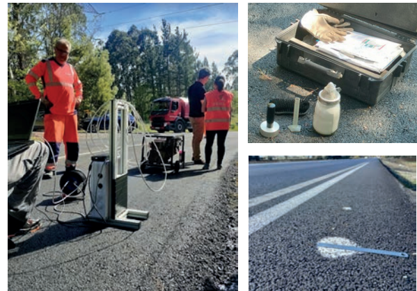
Figure 15c. Details and results of macrotexture measurements with a laser scanner and comparison of results with the sand patch test
