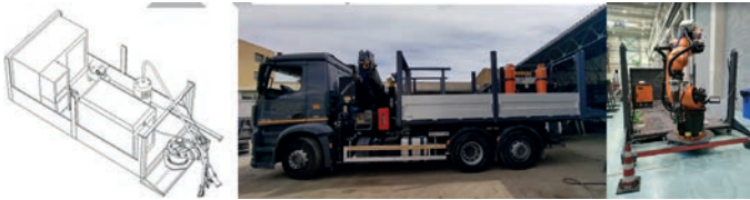
Figure 2. Representation and images of the multipurpose robotic platform.
