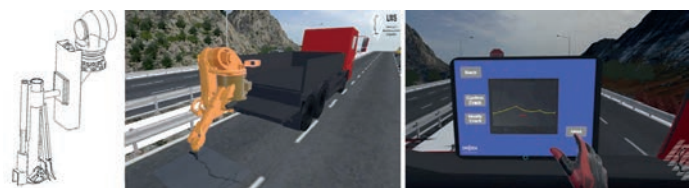
Figure 8. Left: Representation of the sealing tool attached to the robotic arm; Centre: VR footage of the crack sealing process; Right.: In-cab VR monitoring system.
