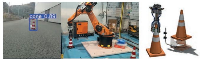
Figure 4. Left.: Cone identification; Centre: Cone placement using the robotic arm; Right.: Representation of the tool for placing and picking up the cones
