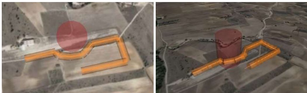
Figure 4.16: A top (left) and a perspective (right) view of the optimal solution in the use case 2. An alternative flight plan for UAS 2 is generated to avoid the geofence.
