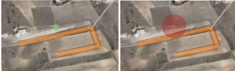
Figure 4.15: Left, top view with the initial flight plans in the use case 2. The Operational Volumes without conflicts are also shown. Right, situation after the detection of the jamming attack. A geofence (in red) is created around the attacked UAS, which generates a conflict with the flight plan of the other UAS.
