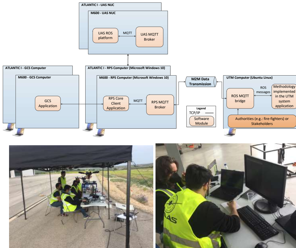
Figure 5.7: Setup for the experiments. On top, an view of the interfaces between the components run on each computer. The computers running the RPS for the two UAS and the UTM system were communicated through the Internet via the MQTT protocol. At the bottom, pictures of the UAS Ground Control Station (left) and the UTM computer (right).
