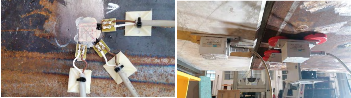
Figure 80. Instrumentation: strain gauges and clinometers
