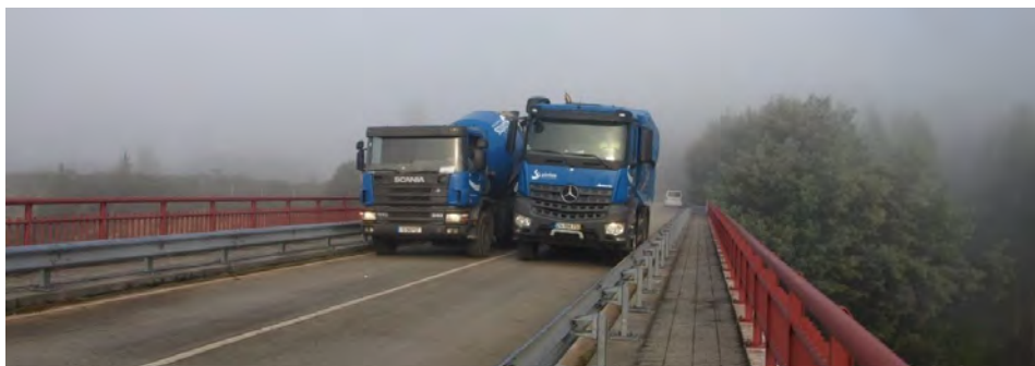
Figure 20. Trucks at the mid span (Load case 1)
