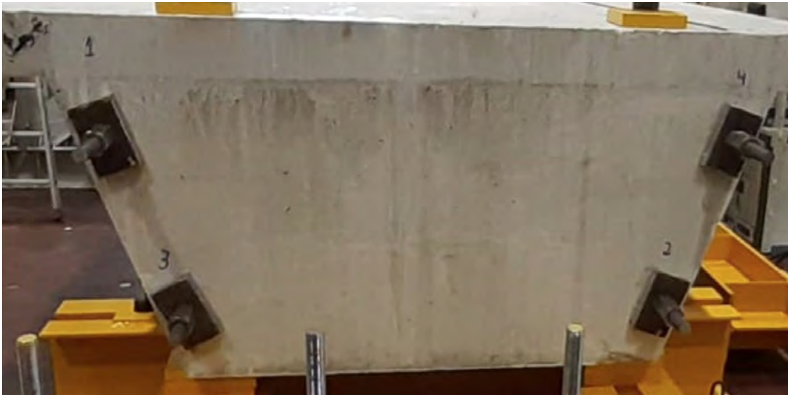
Figure 76. Prestressing the prototype in the laboratory
