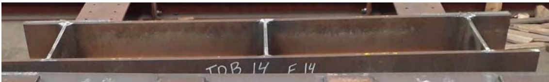
Figure 72. Distribution beam for the hydraulic jack in the test
