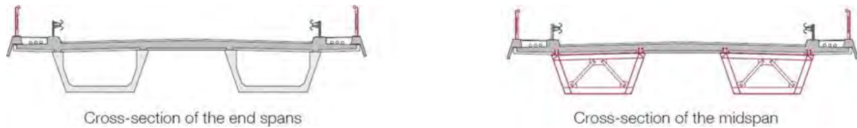
Figure 15. Overpass Cross-sections (Armando Rito, 2012)
