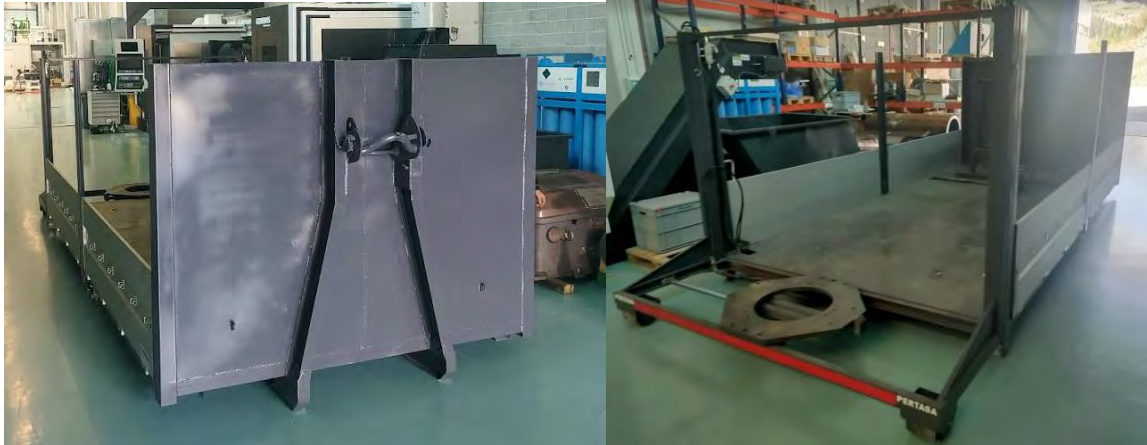
Figure 15. Customized container built for the modular robotic platform.
