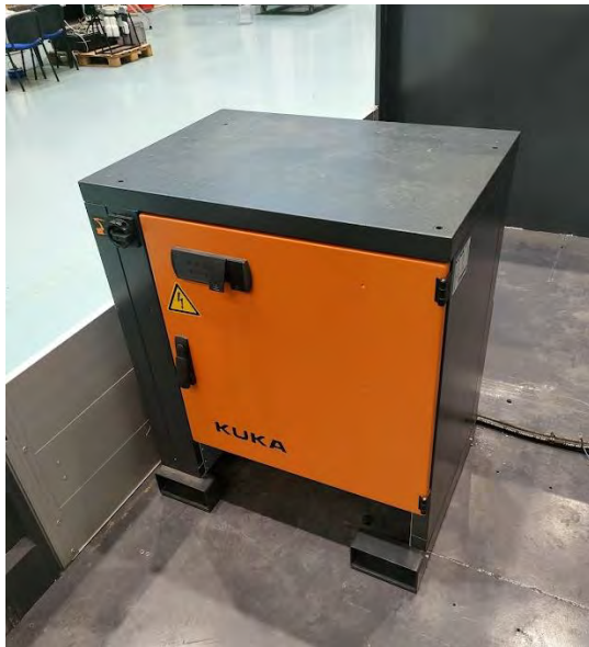
Figure 39. The robot control cabinet fixed to the container
