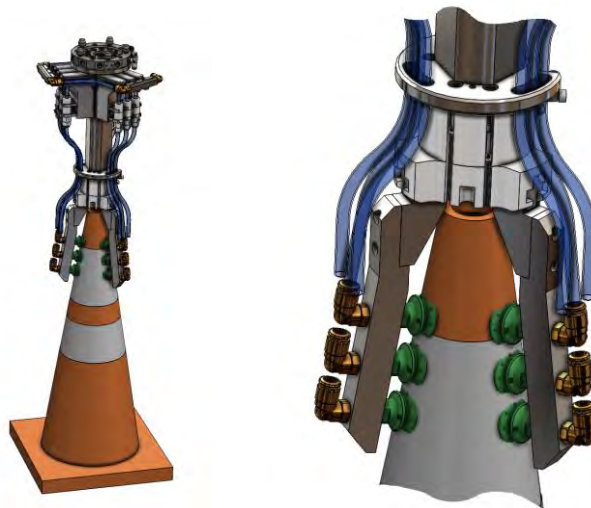
Figure 16. 3D model of the cone handling tool
