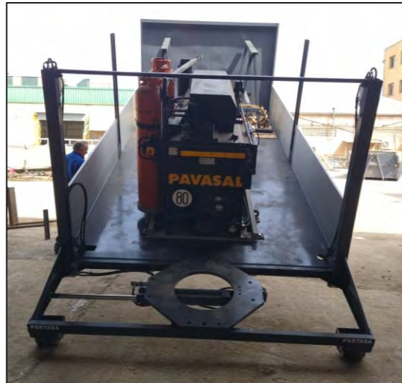
Figure 40. Sealing machine secured to the container.
