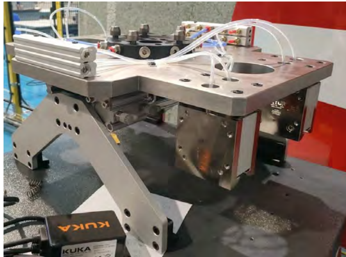
Figure 21. The manufactured safety barrier handler
