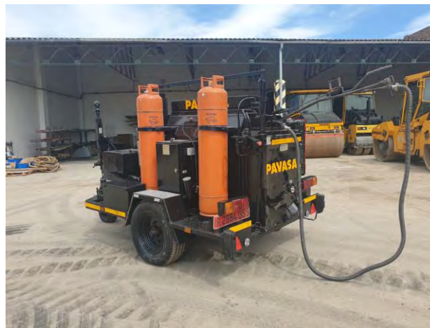
Figure 2 Sealing machine for heating and melting the mastic
