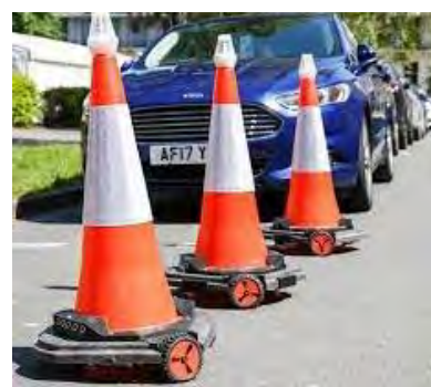
Figure 19. Remotely controlled traffic cones
