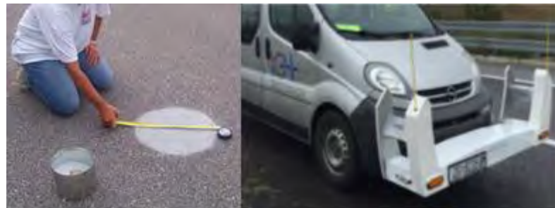
Figure 23. On the left, MTD or sand patch texture detail, as per EN13036-1. On the right, MPD laser profilometer details
