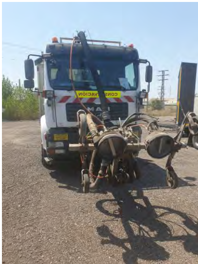
Figure 15. Tool for lane marking removal
