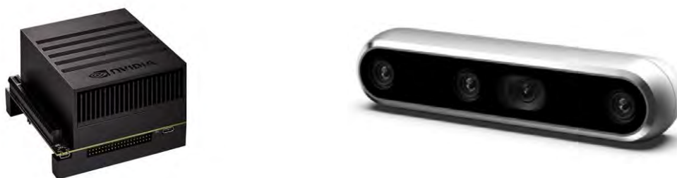
Figure 2: Examples of GPU (NVIDIA Xavier) and RGB-D camera
